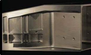
The 6AL-4V titanium housing required machining some features to tolerances as tight as  $\pm 0.001$ inch. To reduce weight, the component incorporates radial pockets, which are visible in the closeup view on the right. When creating these pockets, programmers used GibbsCAM to control profiles, wall thicknesses and surface texture with step-over values.
