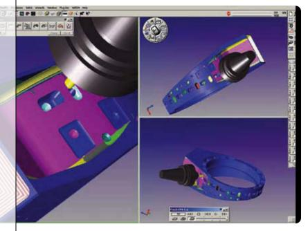
GibbsCAM enables programmers to choose multiple perspectives for display. Here, the Mars Science Laboratory rotor housing undergoes toolpath verification with Cut Part Rendering. For easier visualization of multiple operations, each operation can be displayed in a different color. launch in 2011. In both projects, GibbsCAM CAM software played an important role in the shop's ability to machine these vehicles' complex components to stringent tolerance and surface finish requirements.
