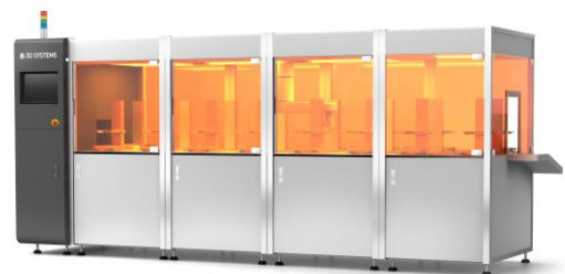
3D Systems' Figure 4 fully automated, high-volume 16-print engine production solution.
