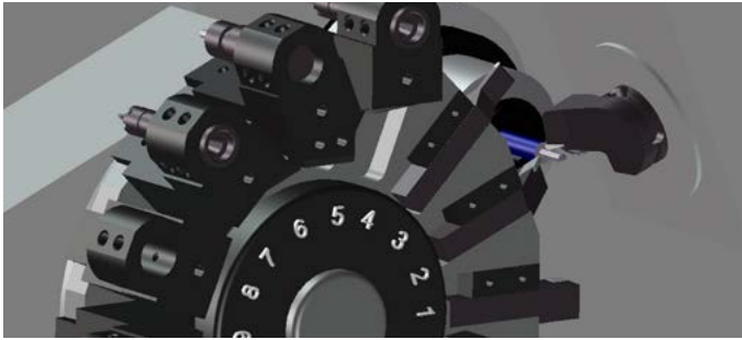
Intermediate tooling provides more accurate simulation of cutting motion.
