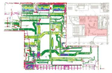
**Figure 2:** The deck analysis from Geomagic Control X shows where the data of the CAD model deviates from the actual conditions on site. This knowledge is used to ensure necessary adjustments are made in good time. Image © MEYER WERFT
