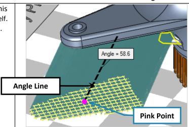
Pick anywhere on the **Angle Line**, a Red Point appear. It is possible to drag it to any direction as well add scaling to the support's section. It is also possible to pick the point at tray level (Pink Point) to move and scale it as well if needed. By doing so, we released the detail so the support won't relay on it on the upper side.
