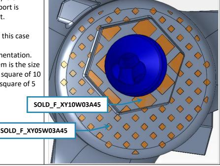
Note on the Table of regions that a bulb was added automatically to indicate that a support was added on this region. The bulb of this region itself is now in **Hide** mode (as this region is no longer required) while the bulb of the relevant support turns to **Show** mode.
