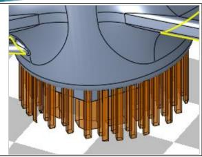
Looking from the bottom (-Z direction) it is possible to see that the first solid support is massive than the second Solid Support.
