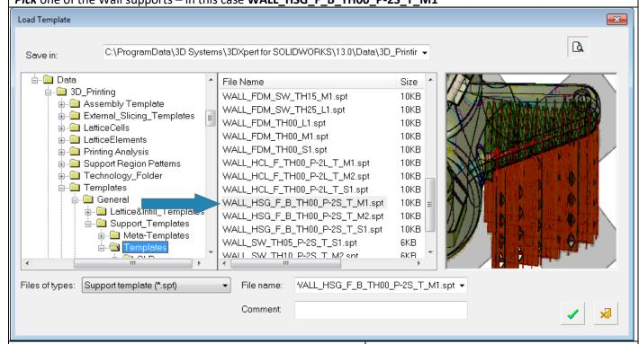
This family of supports can give a very good cover for small up to large regions with a good strength and yet easy to remove due to the "**Teeth**" (**T** in the code name) at the touch points with the part.
