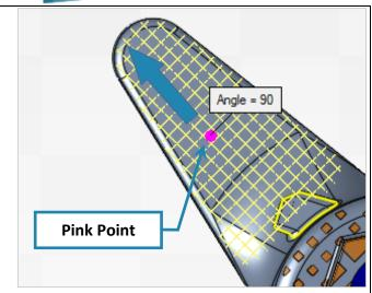
While dragging the Overhang angle is analyzed and result shown on the label attached to the **Angle line**.
