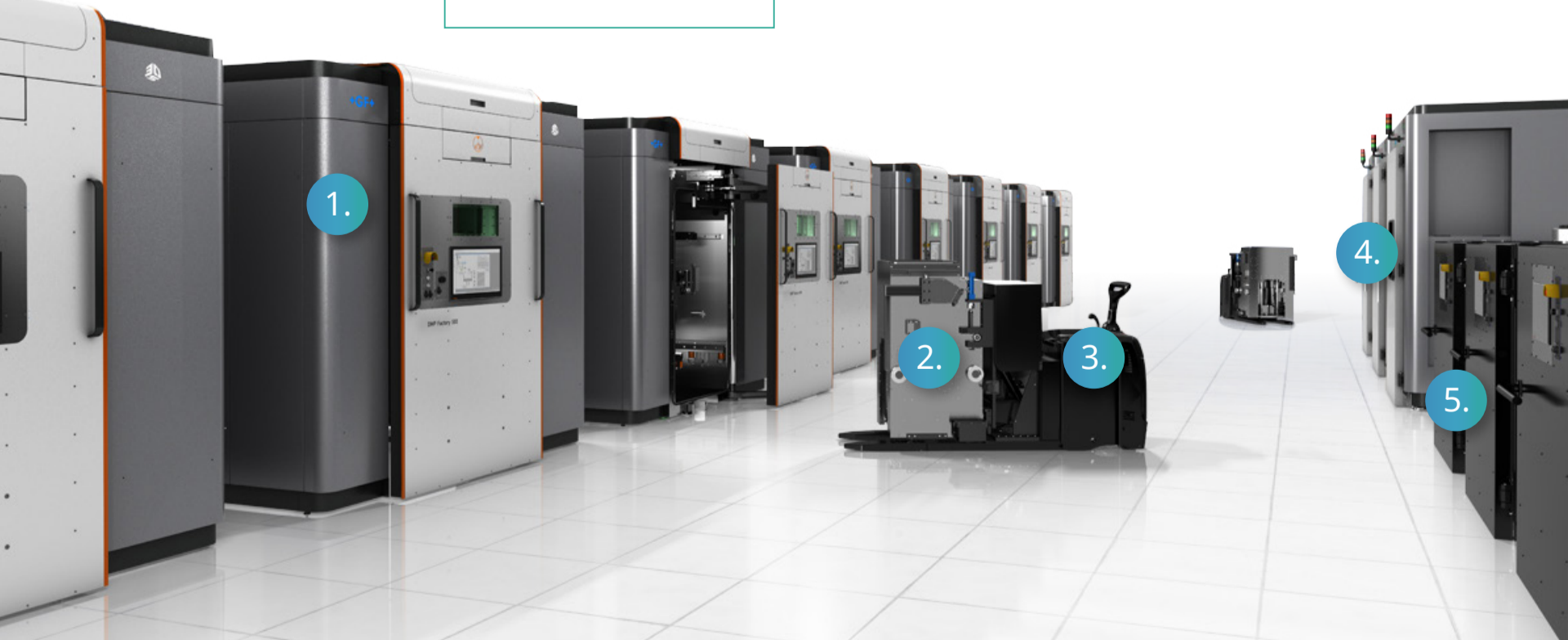
3. Transport Module (TRM) Takes RPMs from PTM to PMM
