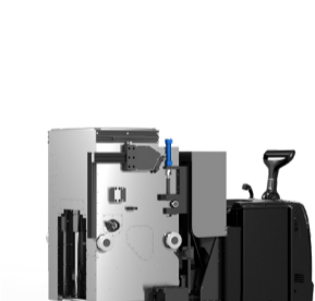
2. Removable Print Module (RPM) Seals the build platform from the atmosphere and moves throughout the factory
