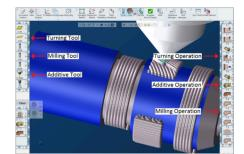
Turning, milling, and additive tools and operations in GibbsCAM 14
